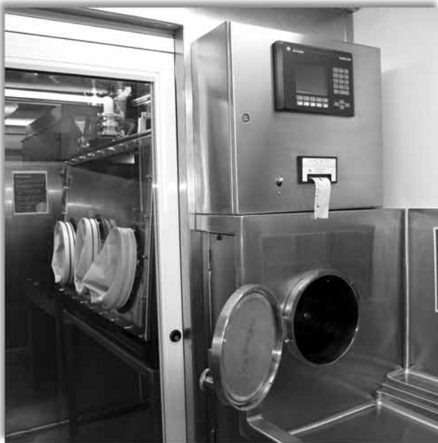
Two-door Autoclave from Glovebox through wall to adjoining lab
